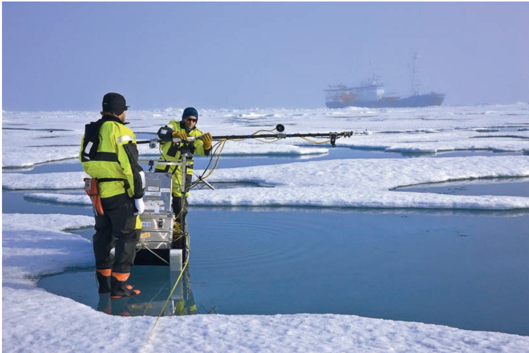
To gain a better understanding of sea-ice loss and heat-transfer processes in the Arctic Ocean as Earth’s atmosphere warms, geophysicists Stephen Hudson and Mats Granskog use several scientific instruments mounted on a sledge to collect data relating to the reflection, absorption, and transmission of solar energy by different types of arctic sea ice and by melt ponds of varying depth on the surface of the ice.
